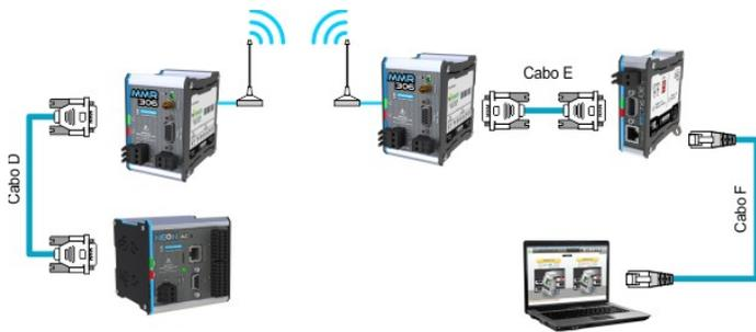
**Cabo D:** Cabo MMR Dados(DB9) – PLC GII/3 COM2 TX7/RX8(DB9) [PN: 302.306.100.000]
