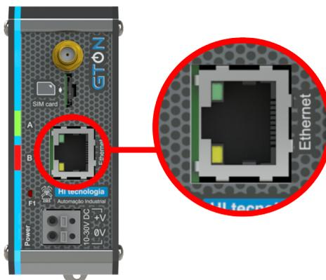
**Conector de interface Ethernet do GTON-M E4G.**
